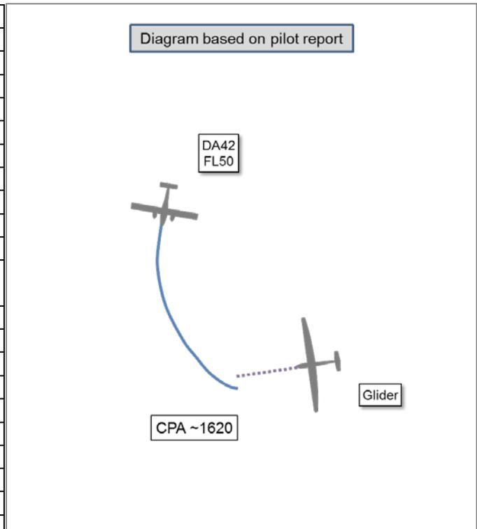
**THE DA42 PILOT** reports that he saw a white glider in the left 1030 position, co-altitude, at a range of ¼nm, in straight-and-level flight and on a converging course. He turned away, and the glider passed close behind. He reported the Airprox to Lakenheath. In subsequent discussion with an Airprox Inspector, the pilot was firm in his assertion that he had reported the Airprox to Lakenheath and that he remembered doing so in light of his previous Airprox, earlier the same day [2015131].
